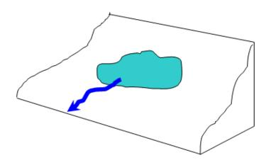
e) **Seep not feeding a stream** – Water is mainly from sub-surface sources where the groundwater discharges onto the surface and includes springs. The seep tends to disappear again as flow dissipated underground and there is no apparent link to any defined watercourses.
