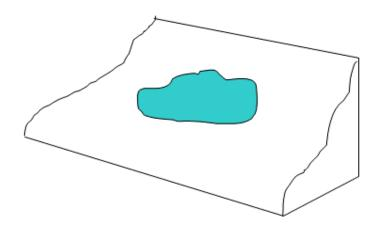
f) Depressions – A basin shaped area that allows for the accumulation of surface water. It may or may not have an inflow or outflow. Water sources include precipitation, sub-surface water as well as surface flows. Depressions tend to accumulate salts and minerals.
