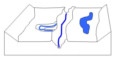
d) Seep feeding a stream – Water is mainly from sub-surface sources where the groundwater discharges onto the surface and includes springs. The outflow is usually via a well-defined channel towards a watercourse. The slope can be gentle or severe.
