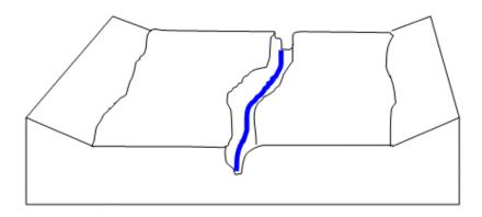
c) **Floodplain** - Can be gently sloped, but generally steeper, resulting in higher surface-flows and a net-loss of sediments. Usually have a clearly defined eroded/developed channel, but with levees and/or depressions outside the main channel. These can include cut-off meandering channels (horseshoes). The flat area outside the channel can also be characterised by alluvial sediment deposits.
